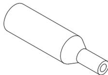
The female IP172 interconnection protector should be assembled on a EAxxx extension cable.
